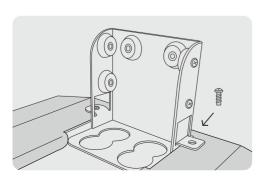
**Step 2:** Place the brackets on the top of the screw holes.
